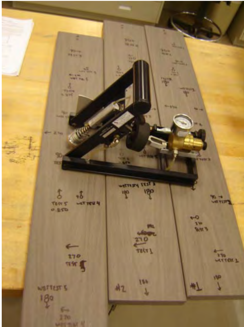
Photo No. 2 ASTM F 1679 Test Setup (Dry Conditions)
